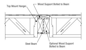
JOIST TO STEEL BEAM WITH APPROPRIATE HANGER **DETAIL NO. 15**
