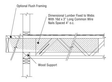
NOTE: Cantilevered Dimensional Lumber must be engineered for load and deflection per applicable code.
