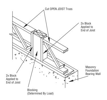
BLOCKING UNDER CONCENTRATED LOAD ON PARALLEL END WALL
