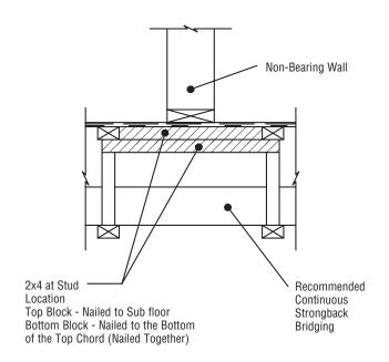
NON-BEARING WALL PARALLEL WITH JOISTS
