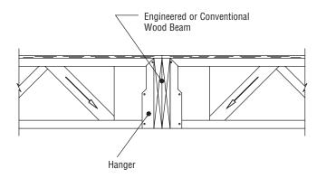
JOIST TO WOOD BEAM WITH APPROPRIATE HANGER **DETAIL NO. 4**
