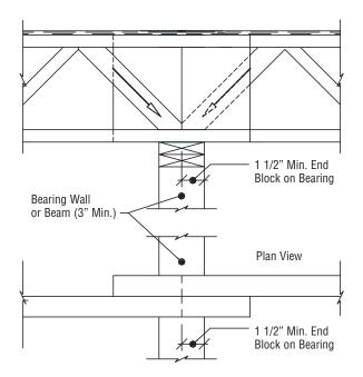
OVERLAPPING ON INTERIOR BEARING **DETAIL NO. 3A**
