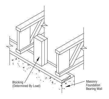
BLOCKING UNDER CONCENTRATED LOAD THAT FALLS BETWEEN JOISTS
